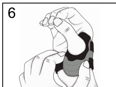
6: With your thumb relaxed, squeeze the aluminum stay to custom fit the brace to your thenar contour.
